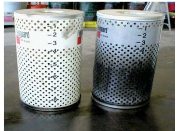
Fuel Filter after clean-up run with the new formula.
