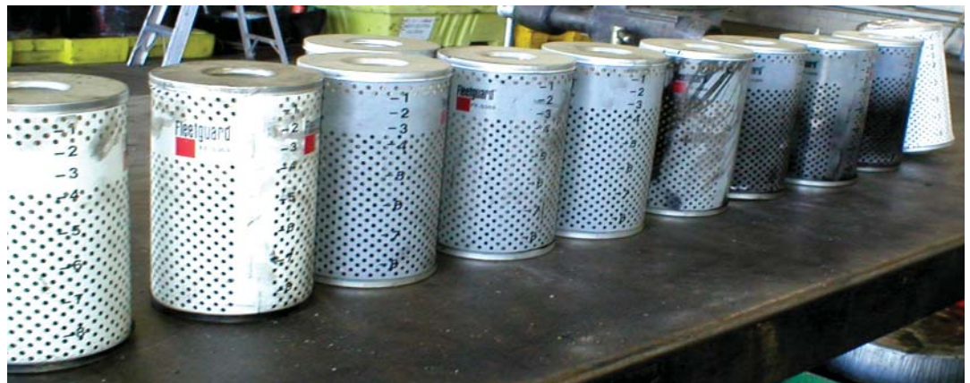
Brand New Filter is seen on the far right of picture. The next filter (second on far right) has been contaminated by Black Filter Syndrome. The continued use with the new formula will clean-up the Black Filter contamination resulting in prolonged filter life and therefore critical engine protection.
